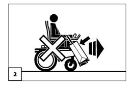
Before maintenance work as well as alterations, attachments and adjustment on the electric vehicle, the drive mode is to be selected and the vehicle switched off. – Danger of accidents due to unintentional motion of the vehicle!
