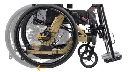
**90 mm adjustment for great stability** The wheel footprint automatically increases by 90 mm when the wheelchair is tilted.
