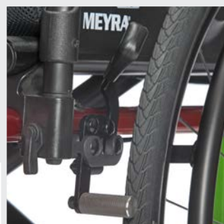
Unique brake with extremely low actuating force
