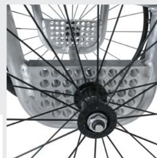
Wheel position and seat height rear variable in 15 mm increments
